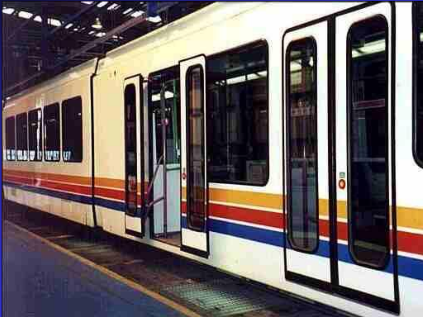
Sheffield tram with plug doors. The leading doors are shown closed and are flush with the body. The rear doors are in the open position.
